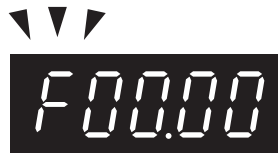
Figure 5.47 Ready for Setting Speed Reference
